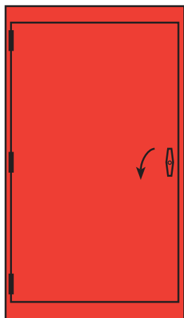
Showing LH T-Handle (Anti-clockwise to open)
