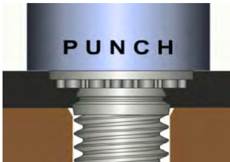
Clinch fasteners require pressing into sheetmetal
