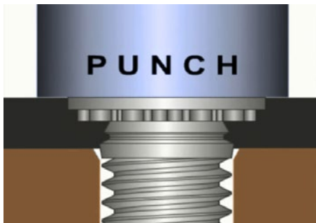
Clinch fasteners require pressing into sheetmetal
